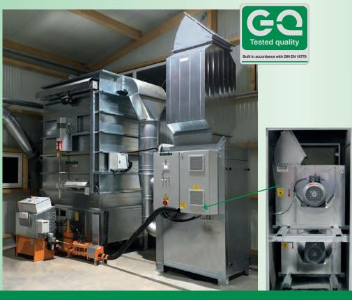
Quiet operation is guaranteed by **noise-insulated fans in** a range of different power classes 2 x 5.5; 2 x 7.5; 11 or 15 kW
