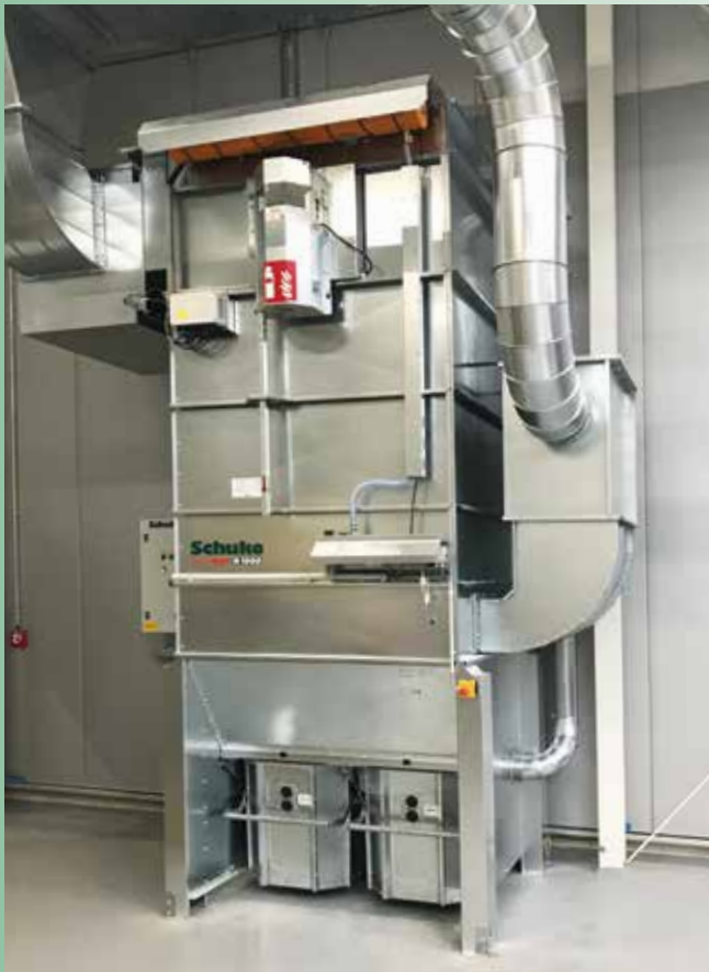
Vacomat N-1000 with a filtering surface of 50 m 2
