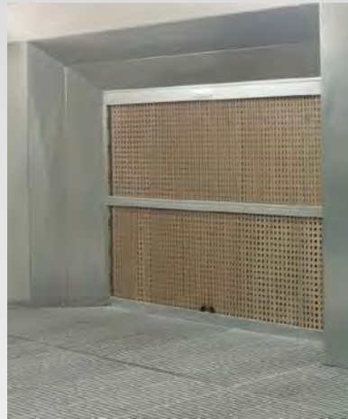
The efficient combination of a paint spray mist extraction wall and an underfloor extraction system
