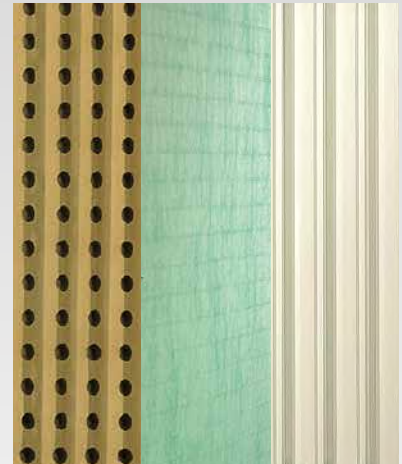
Baffle surfaces made of cardboard, filter fleece or steel ribs for dry separation
