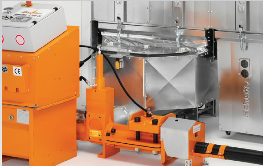
Dust extractor VACOMAT with chip collector SPB 50 and briquetting press Compacto 700
